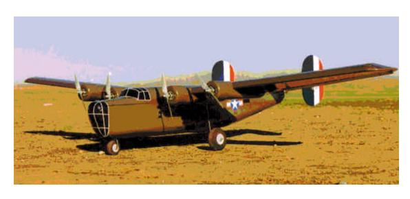
rudder, elevator, ailerons, and throttle. It weighs 64 ounces and has 460 square inches of wing area. The four motors are wired in parallel, and draw about 44 amps. With 5.5x4.5 APC propellers, they produce 30 oz. of thrust. Since this wonderful photo op (Courtesy of Rob Askegaard), Jerry has installed 3 bladed 5 x 3 props all painted up black with yellow tips. That really looks great!
