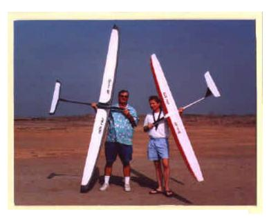
My first attempt to build this plane using a true RG15 airfoil @ 8.9% thickness resulted in a plane which could fly extremely fast but had very poor slow speed flying characteristics. The plane was forever falling out of the sky due to tip stalling.
