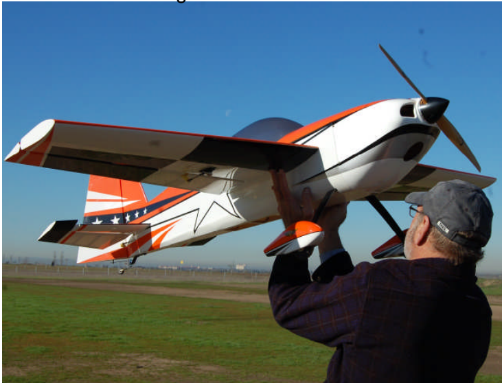
Bret Bayless and his 3-D Hobby Shop Extra/AJ Slick. 71" span, Hacker 850 motor and an 18 x 10 prop.
