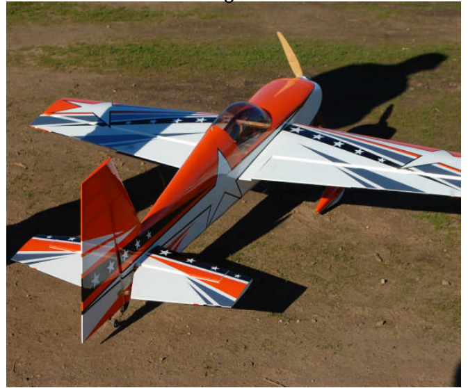
Bret Bayless and his 3-D Hobby Shop Extra/AJ Slick. 71" span, Hacker 850 motor and an 18 x 10 prop.
