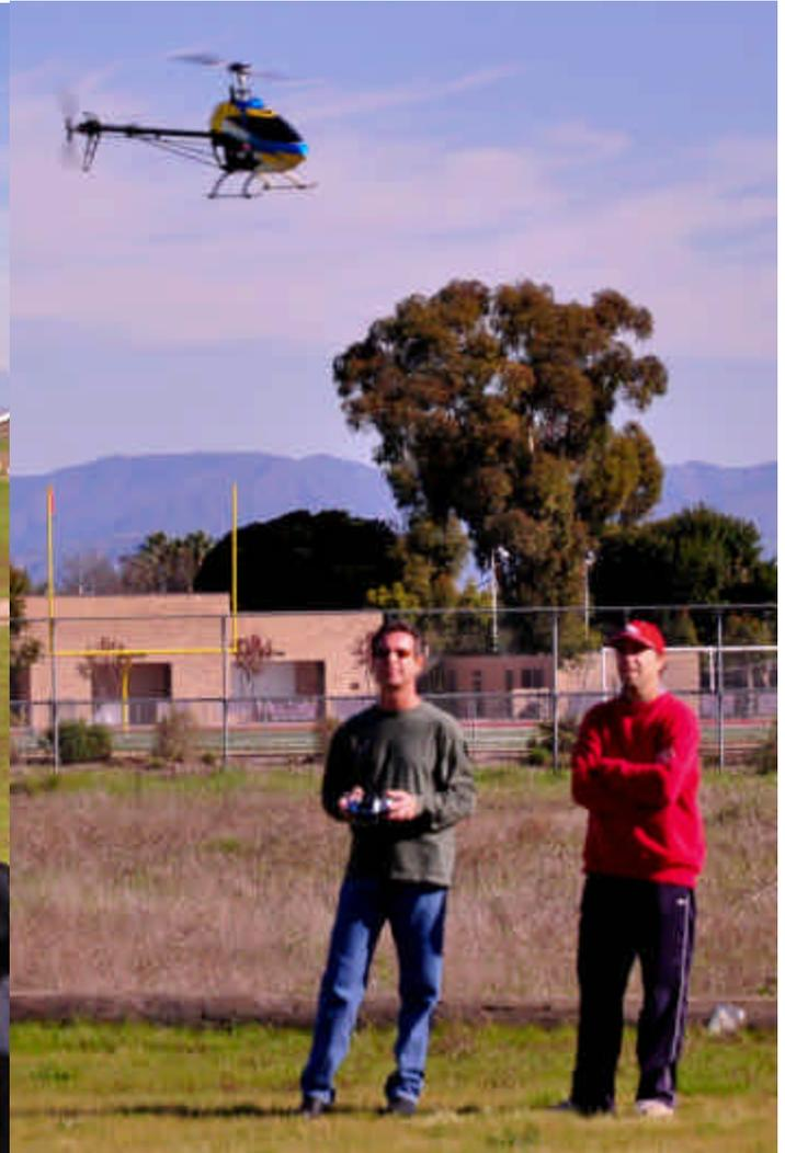
Member Alex Beller (left) flying his Logo 600, a German helicopter set up with 3750 mAh LiPos in a 12s configuration swinging 600 mm blades. Alex can get about 10 minutes of flight time on this heli. Member Joe Bushor looks on.
