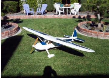
Astro 60 with super gear box Astro 204 Speed Control (12 lipo cells max) Prop 24x12 – 31 Amps, 1300 watts 4- HS475HB Servos Spectrum AR6200 receiver
